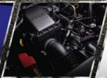
1.5L* 4 Cylinder, In-line, 16 Valve DOHC, Chain Drive with Dual VVT-i Engine
