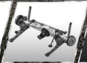
4-link with Lateral Control Rod rear suspension
