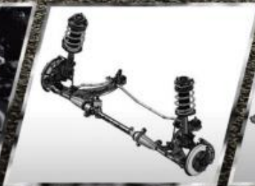
MacPherson Strut with stabilizer front suspension
